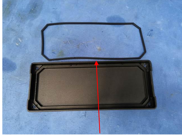
Waterproof gasket was used
