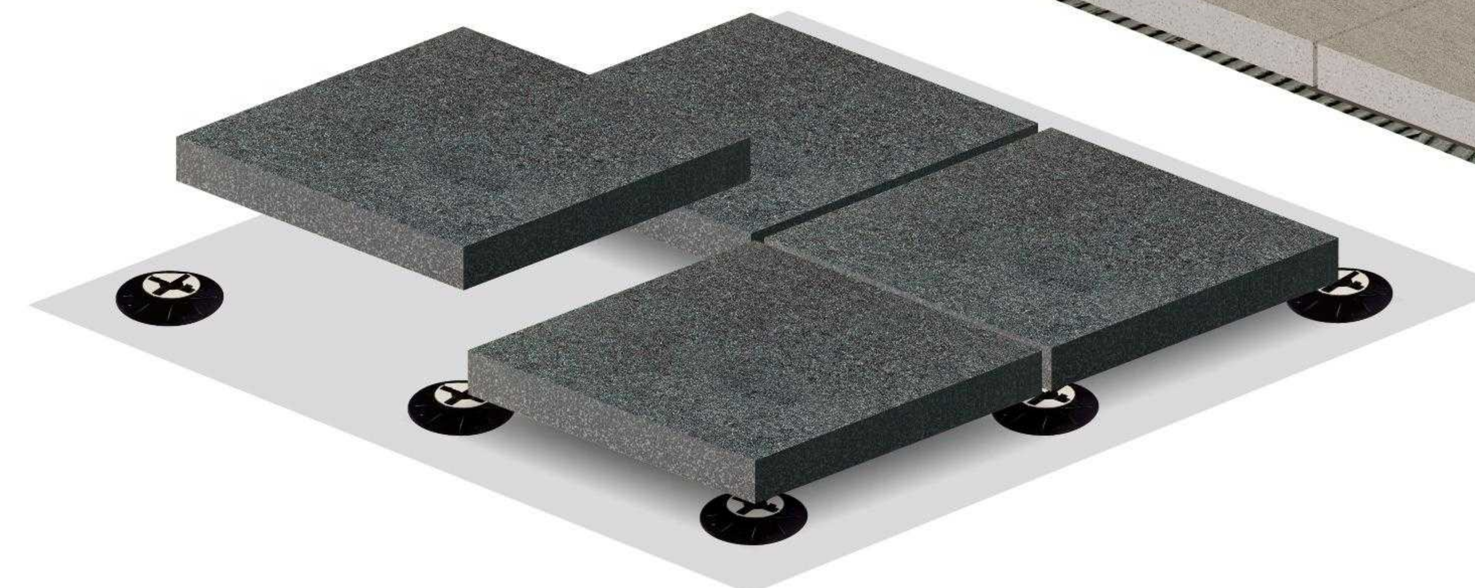
Laid on pedestal
