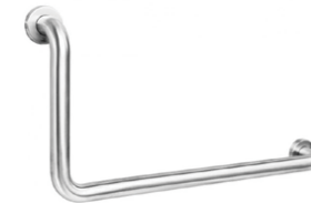
EPGB-L32-36 Grab bar 12"x24" Material Thickness SUS 304 Stainless Steel 300x600mm Satin 90° OD 32mm 304
