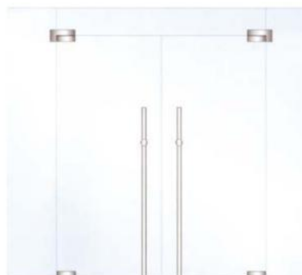
Double Door Installations Require Two Locking Handles
