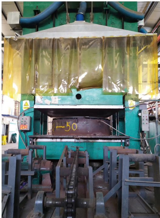
3600 tons of super large flat plate vulcanizer in BAYTAIN
