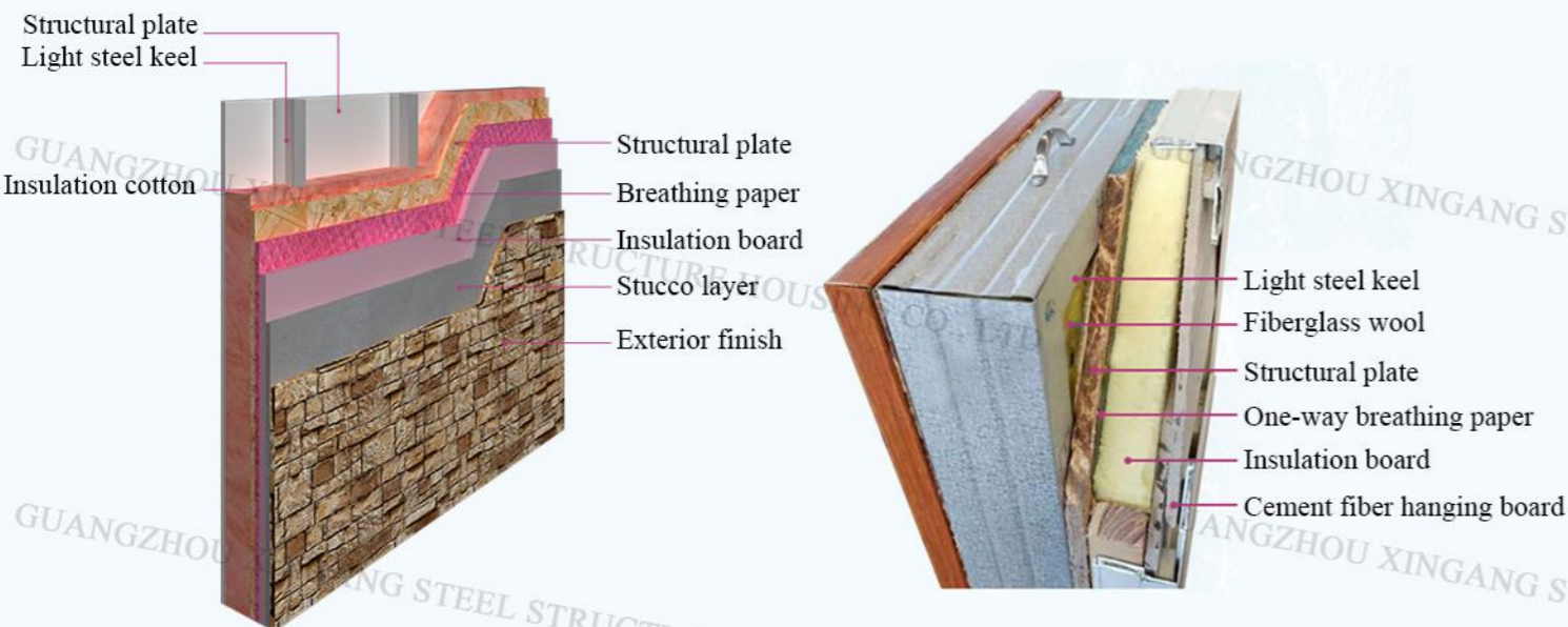
THE OVERALL STRUCTURE OF THE INNER AND OUTER WALLS
